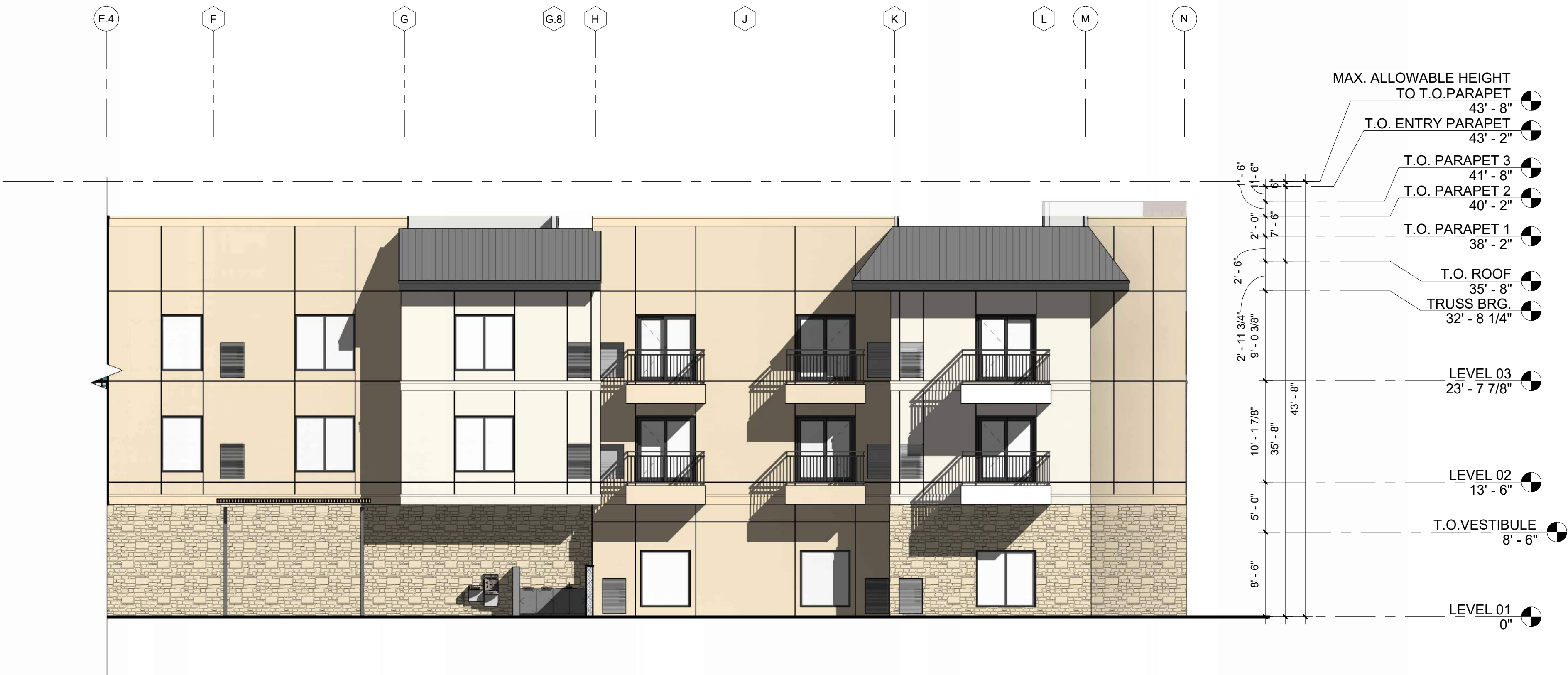
2 NORTH-EAST ELEVATION - PARTIAL A-4.3 SCALE: 1/8" = 1'-0"
