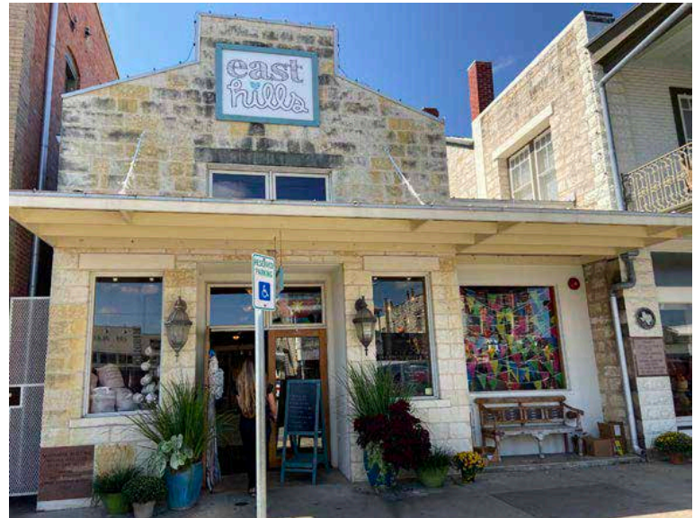
Figure 3-64. Example of an appropriate new commercial infill building at 127 E. Main Street, constructed with the front wall flush to the sidewalk – consistent with the adjacent historic buildings on Main Street east of Milam Street. Source: City of Fredericksburg Historic Preservation Office.
