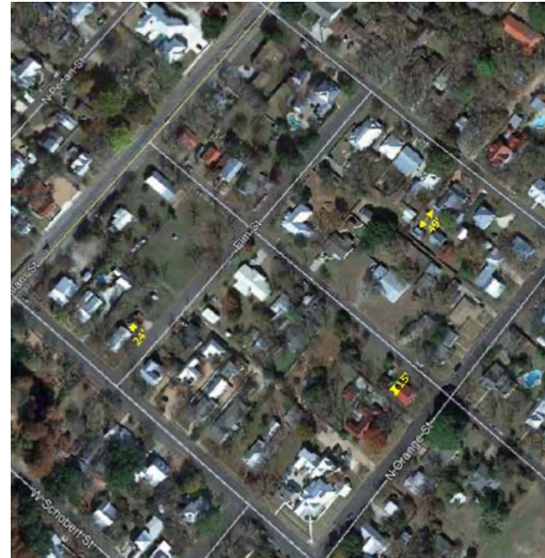
Figure 3-57. Aerial photograph showing a sampling of setback measurements between historic main houses and historic accessory buildings within the Fredericksburg Historic District. Note a range of setbacks between 15 feet and 66 feet. Source: Basemap and measurements from Google Earth Pro.
