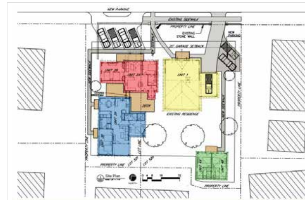
Figure 3-59. Example of an inappropriate site plan on E. Travis Street that proposes lot coverage far denser than the surrounding neighborhood. Note the contrast in setbacks between the proposed buildings and the surrounding historic buildings. Note also the proposed inappropriate parking location on the main street, with no buffering or landscaping. Source: City of Fredericksburg Historic Preservation Office.
