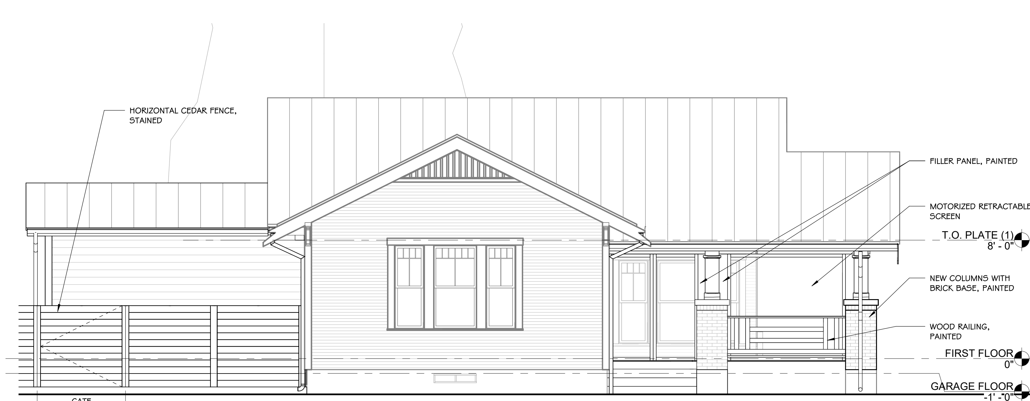
04 EAST ELEVATION SCALE: 1/4" = 1'-0"
