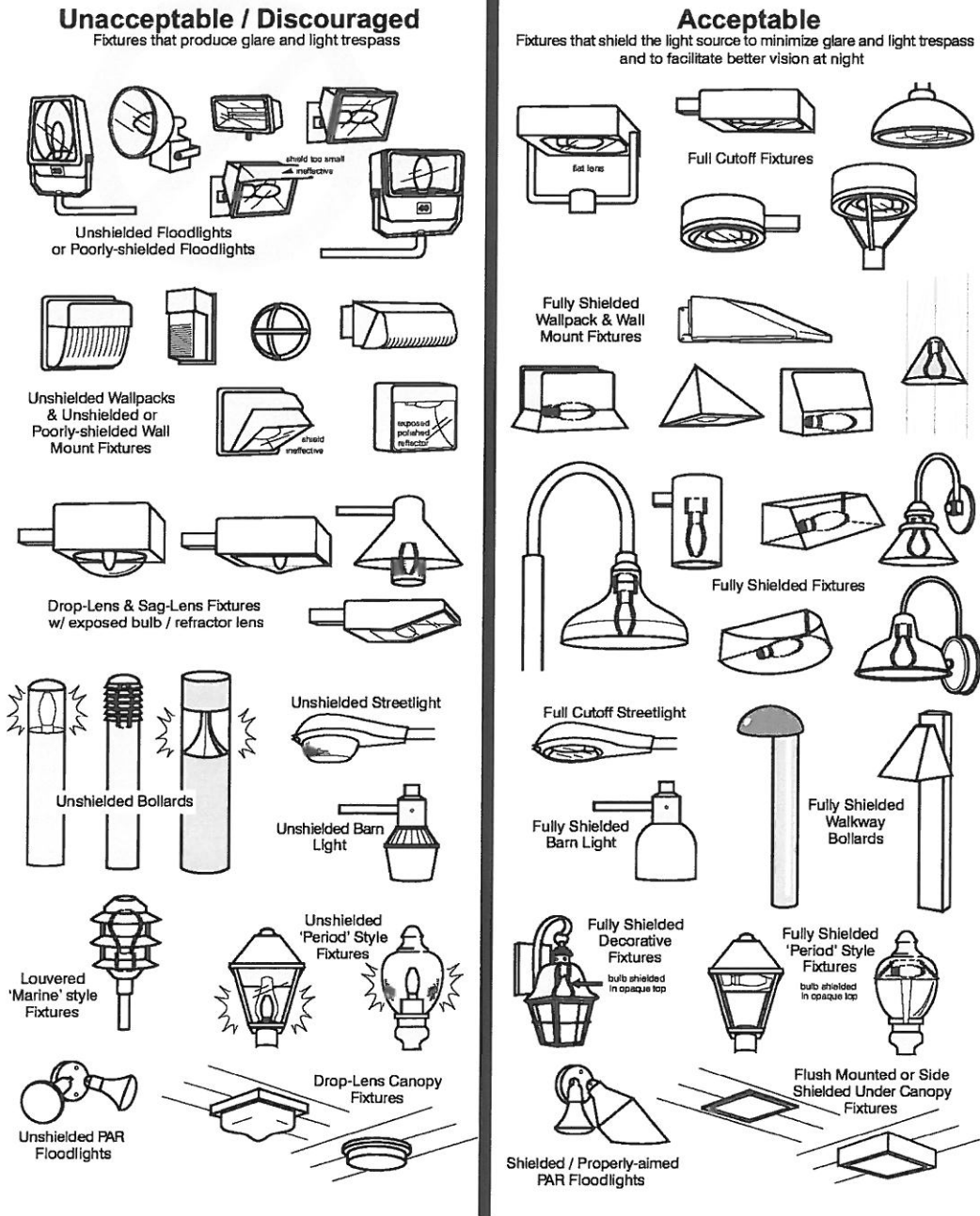
Figure D: The lights on the left are non-conforming due to inadequate shielding. Those on the right can be used in most cases; however, the mounting height and proximity to the property line may require additional shielding to prevent the luminous elements from being visible from any other property.
