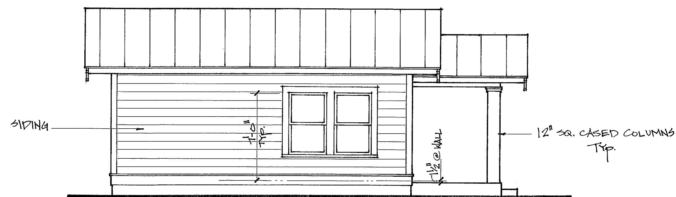
LEFT SIDE (EAST) ELEVATION 1/4" = 1'-0"
