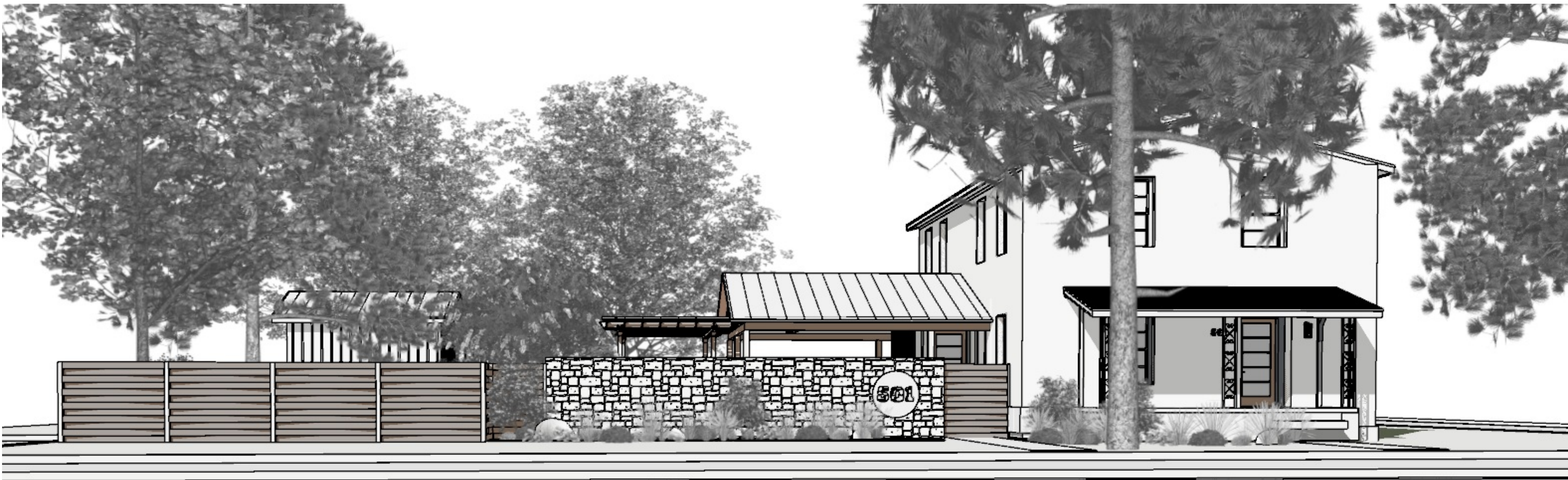
PROPOSED ENTRY DOOR PAINTED WOOD TO MATCH TRIM 5 PANEL TO ALIGN WITH HORIZONTAL WINDOW LITE PATTERN; GLASS TOP 2 PANELS, SOLID BOTTOM PANELS.
